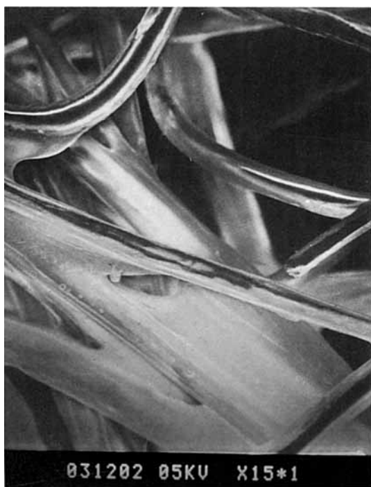
Figure 3 SEM of surface of polyacrylate-bonded jute/polypropylene blended (80:20) nonwoven ( \times 150 ).
